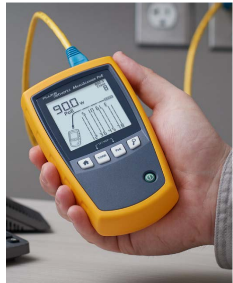
Figure 4. The MicroScanner™ PoE displays the class and power level as reported by the switch.
