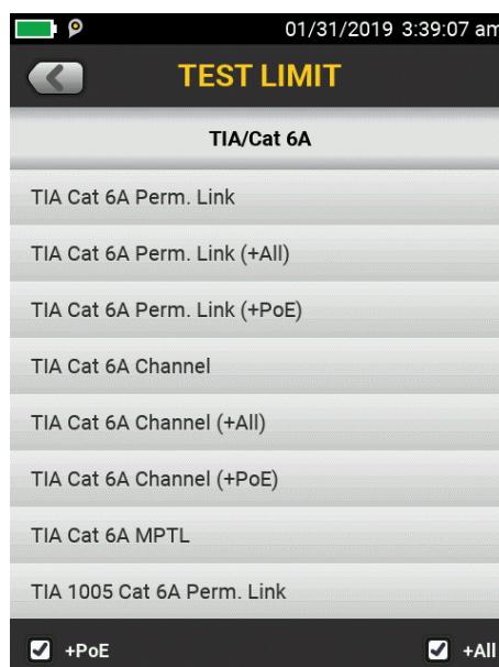
Figure 3. By selecting “+PoE tests in the DSX Series, a complete set of resistance measurements are made on the link to ensure proper PoE operation.
